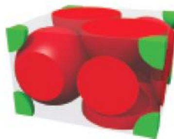
(c) Unit cell of TiO_2 , the rutile structure
